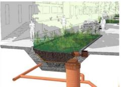
The photo on the left shows the flooding in Uppsala Travel Centre in the summer of 2018. The picture on the left is a sketch of how stormwater beds handle and purify rain water.
